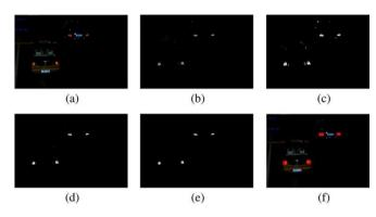
Fig. 4. Example of the rear-lamp localization process. (a) Input image. (b) Converted rear-lamp color image. (c)–(e) Binary images obtained by three thresholds ( $\sigma$ 1 = 20,  $\sigma$ 2 = 40,  $\sigma$ 3 = 80). (f) Rear-lamp localization results.
